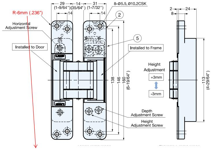
Note: There will be a slight difference in the corner radius on these hinges compared to the mortis that the template produces. The hinge has a 6mm (.236") radius on the corners; when you produce your mortise with a 1/2" cutter, (.250" radius) there will be a slight amount of hand work needed in the very corner of the mortis pocket.
